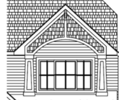
Flared columns with varying style of shake detailing
